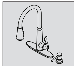
Option 1: 4 Hole With Deckplate Installation
