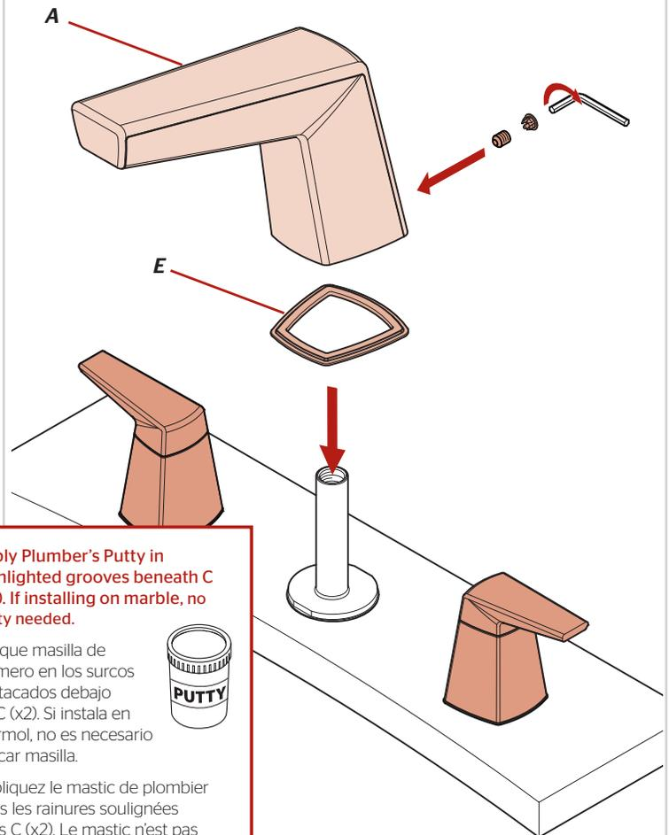
Apply Plumber's Putty in highlighted grooves beneath C (x2). If installing on marble, no putty needed.
