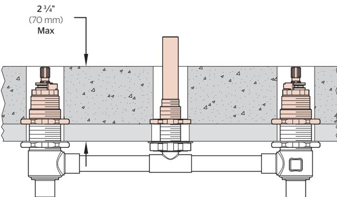
If deck thickness exceeds 1 3/8" (35 mm), Pfister™ Stem Extension Kit 974-375 must be used.
