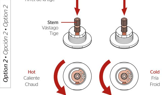
Stem Stop can be inserted into Stem in either of two ways, depending on the rotation you want to have for your handles.
