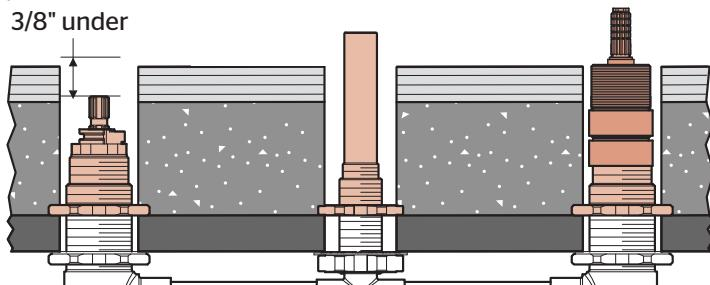
**!** Two Pfister™ 974-375 Stem Extension Kits must be used. Sold separately. Trim will not work if stem is located more than 3/8" below the deck and more than 1/8" over the deck.
