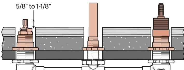
**!** Pfister™ Stem Extension Kit 974-375 must be used. Sold separately. Trim will not work if the stem height is less than 5/8" and more than 1-1/8".
