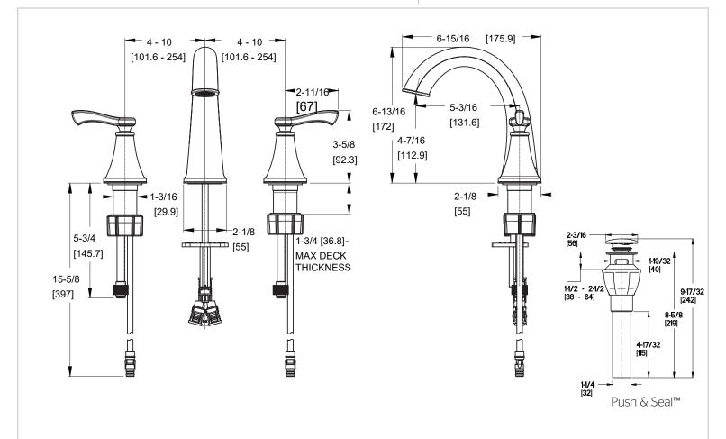
Ø1-1/4 Min to Ø1-1/2 Max. Deck Hole Openings
