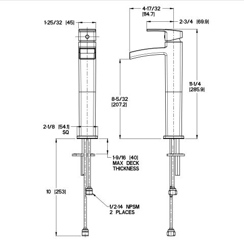
Ø1 Min to Ø1-1/2 Max. Deck Hole Openings
