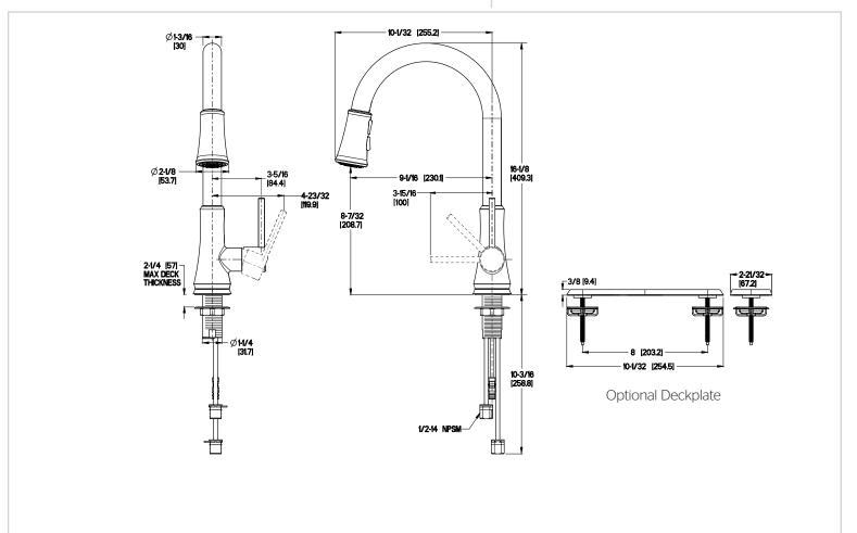
Ø1-3/8 Min to Ø1-1/2 Max. Deck Hole Openings
