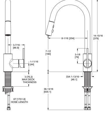
Ø1-3/8 Min to Ø1-1/2 Max. Deck Hole Openings
