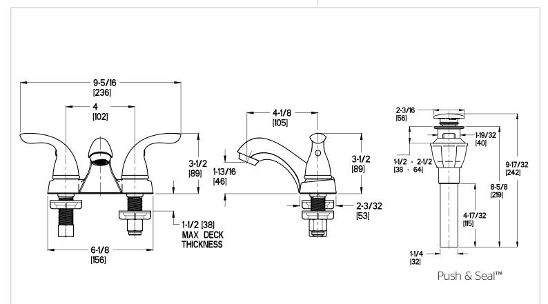
Ø1 Min to Ø1-1/2 Max. Deck Hole Openings
